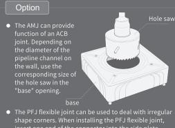
The PFJ flexible joint can be used to deal with irregular shape corners. When installing the PFJ flexible joint, insert one end of the connector into the side plate (approx. 3 lattice) to allow the PFJ to be perfectly integrated with the AMJ.
